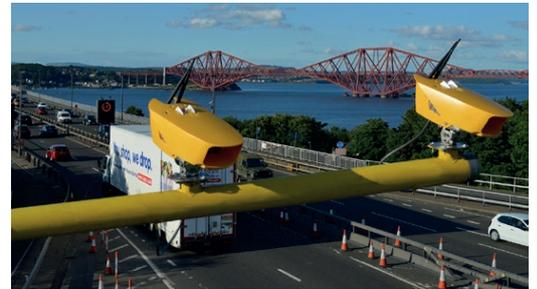
Similarly, video technology can be used to monitor bus lanes. The technology identifies the type of vehicle, either using a 'white list' of approved vehicles or using automatic classification tools. If it is not a bus, the camera will record that it is in the bus lane, supported with an accurate time stamp and a video clip of the violation taking place. It can even reliably identify the difference between, for example, a bus lane and parking lane beside it.
