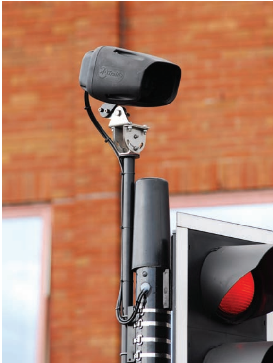
ABOVE ANPR (Automatic Number Plate Recognition) camera in Buckinghamshire. Photo courtesy of CA Traffic
